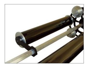
LOAD SMALLER ROLLS ON THE MODIFIED HOLDER.
