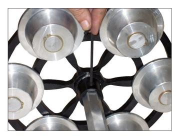
SET LOCK NUT ON LEFT SPINDLE.
