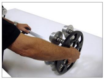
ADD RIGHT SPINDLE WITH SPRINGS AND TIGHTEN WITH LOCKING NUTS.
