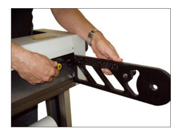
ATTACH LEFT AND RIGHT SUPPORT ARMS TO THE PLOTTER WITH THE SUPPORT ARM SCREWS.
