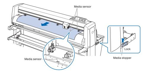
**6** Position the media and the push rollers to correspond with the width of the media.
