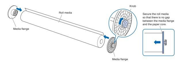
*3* Load the roll media on the stock shaft so that the tip of roll media is facing upward.
