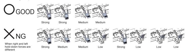
When using three push rollers
