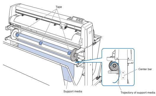
**6** Hold the center portion of the media guide and pull it along the groove in the media guide bracket.
