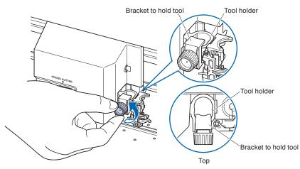
2 While pushing up the tool holder, push until its flange completely touches the upper part of the holder.
