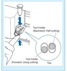
*3* Make sure that the tool bracket is engaged mounted firmly over the flange, and then tighten the screw.
