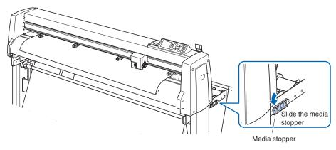
8 When the set lever is up (and the media is held down by the push rollers) and the media stopper is unlocked, pull out the roll media and give it slack.
