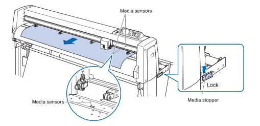
**5** Position the media and the push rollers to correspond with the width of the media.
