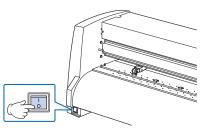
2 Connect one end of the provided power cord to the FC9000 AC line inlet and the other end to an electrical socket of the rated supply voltage.
