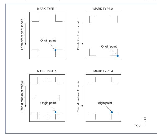
The shapes (patterns) of the registration mark the plotter can scan are following 4 types.
