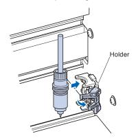
2 Once the pen is attached, releasing the holder fixes the pen in place.
