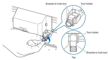
2 While pushing up the tool holder, push until its flange completely touches the upper part of the holder.
