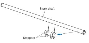
2 Slide the stock shaft into the media stocker. Make sure the stock shaft touches the roller.
