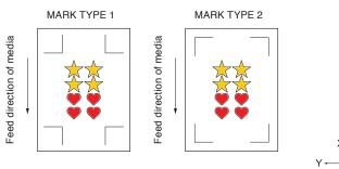
2-2 Create cut design for printing and cutting.It is recommended that cutting data be created by specifying a color that is not used in print data.
