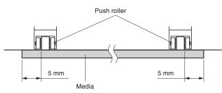
6 Pull the media taut to make sure that there is no slack in the conveyance path, and then raise the media set lever to lower the push rollers.
