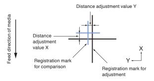
**9** Using the scanned registration mark for adjusting, measure the distance of how much the comparison registration mark needs to be moved so both will overlap, and record the value. As an example, in the figure above, it needs to move in negative directions for both X and Y directions, so both of the adjustment values will be a negative values.
