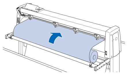
**4** Lock the media stopper (Raise while pulling forward) and pull it out evenly so that the roll paper is straight. Please load so that the roll paper always rests on the media sensor.
