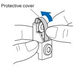
**4** Attach the replacement cross cut unit, and tighten the screw to hold it in place.
