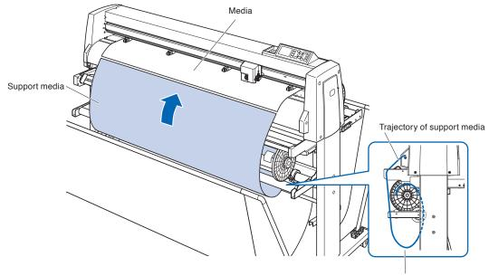
At this time, the support media is in tension state.
