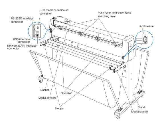
AC line inlet ...... Inlet where the power cable is connected.
