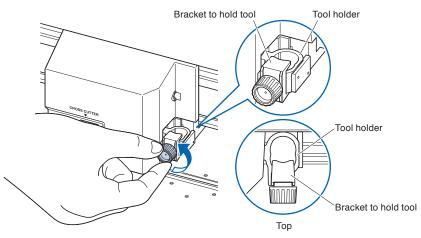
2 While pushing the tool holder in the upward direction, push the Pouncing tool all the way into the holder until its flange contacts the upper part of the holder. The flat edge must be parallel to the tool holder.
