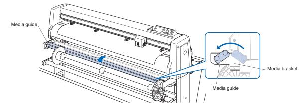
**7** Pull up the support media to the machine's cutting mat surface.
