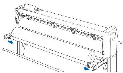
*3* Push the tip of the roll media forward from the back of the FC9000. Make sure to pull it so that there is no slackening across the roll media's route.
