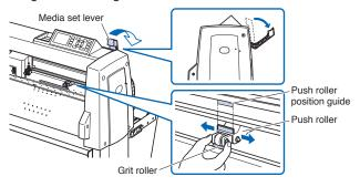
For models with three or more push rollers, place the push rollers other than both ends on the grit roller.
